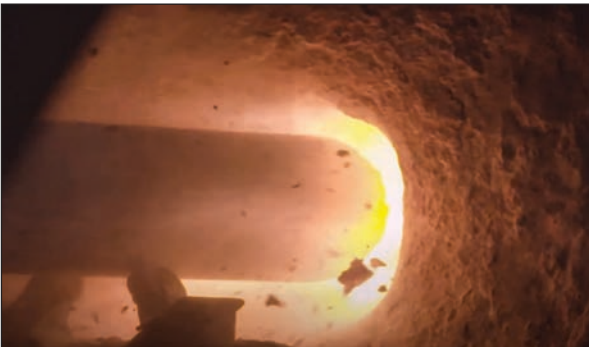
An EarthGrid plasma boring torch cutting through limestone. Photo credit: EarthGrid
