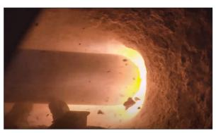
An EarthGrid plasma boring torch cutting through *limestone*. Photo credit: EarthGrid
